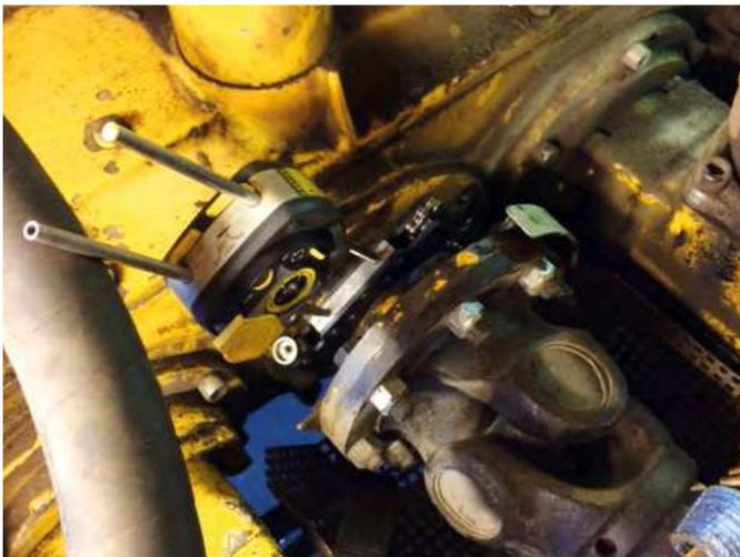
Checking the alignment of the flange parallelism
