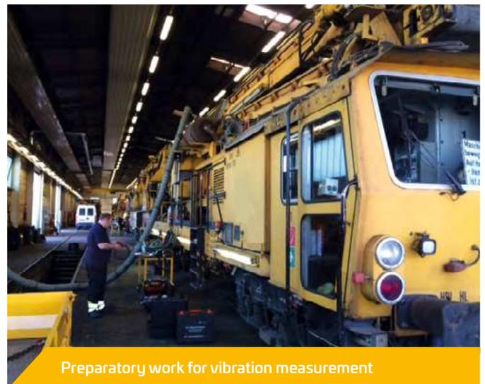
OHP Services was contacted again by the customer and performed a repeat measurement to determine the continued presence of high vibrations on the engine. Finally, field balancing was then carried out.
