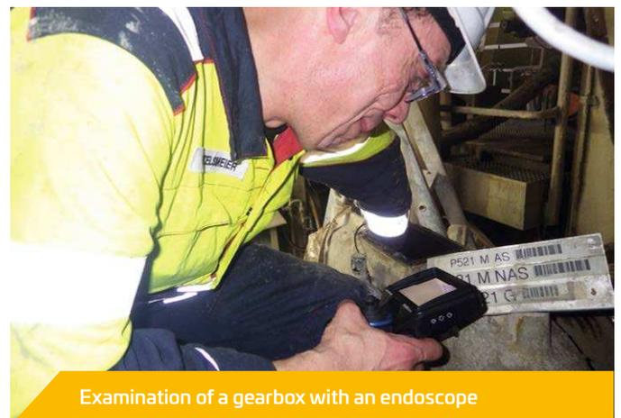
Examination of a gearbox with an endoscope
