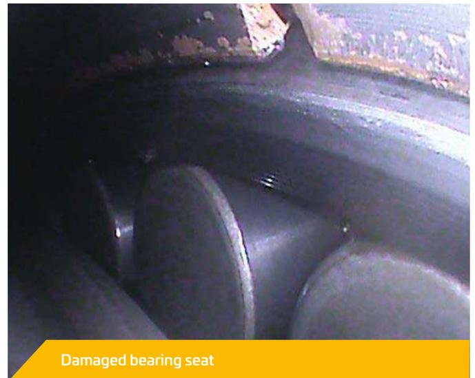
Damaged bearing seat
