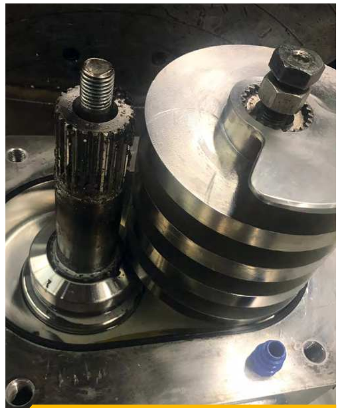
Bearing damage of a spiral pump
