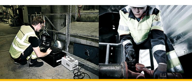
High-tech analysis is the application of specialised technologies to determine the root cause of problems within a powertrain system. Appropriate technologies are selected depending upon the individual (customer) system requirements. These include: vibration analysis, endoscopy, thermographic measurement, balancing, alignment check.
