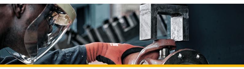
Even components of the highest quality will not perform as designed if they are not installed and adjusted correctly. Misalignment leads to axial and torsional vibrations, overheating, excessive component wear and reduced powertrain lifetime. Energy losses above 10% are a common occurrence in misaligned multicomponent powertrain systems.
