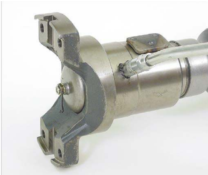
Fig. 3 Grease appears from vent hole
