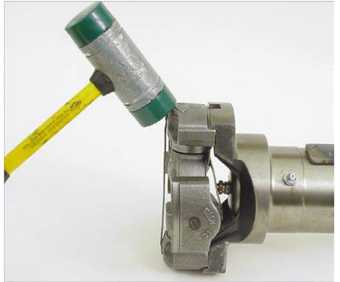
Fig. 2 Opposite bearing installed
