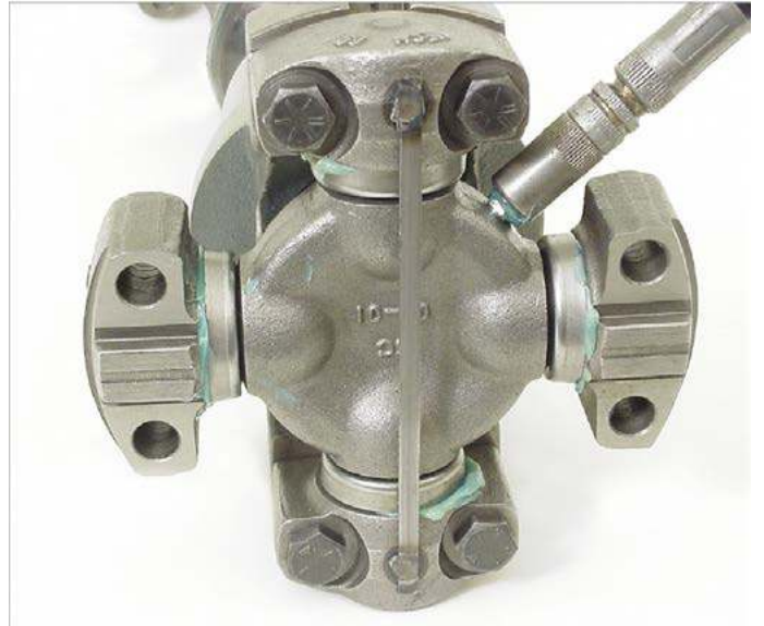
Fig. 4 Seals allow grease to bleed so lubricant can flow through all trunnions
