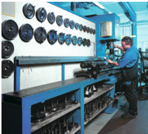
Pre-adjustment of the driveshaft on specially-designed straightening presses.
