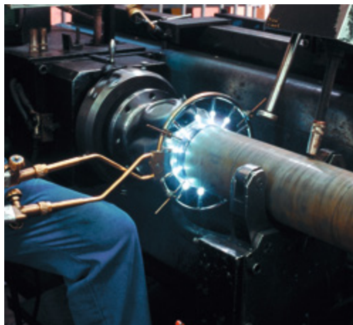
In some cases the driveshafts are being preheated after the compression. This is to prepare them for the welding seam.
