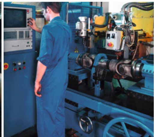
Computerised balancing technologies guarantee faultless performance of the Cardan shaft.
